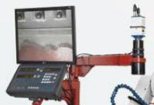
The cutter measuring device is directly online with the PLC of the machine.
