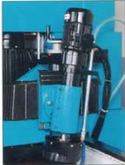
ANGLE ADJUSTABLE OF FINE GRINDING ATTACHMENT
